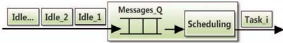
Fig. 1. The Monolithic Scheduling architecture. Task request messages are passed to the scheduler and enter a message queue, where they wait until they are assigned to an idle process.
